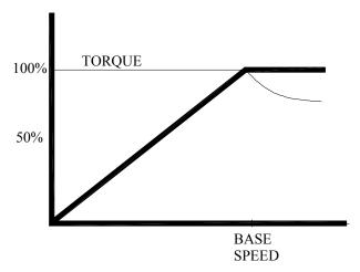
With a variable speed controller using solid state devices, the torque is also limited by the current ratings of the devices. A new torque speed curve applies as shown here on the left. The dark line shows horsepower available. At half speed, although delivering constant torque, the motor only develops one-half horsepower.
