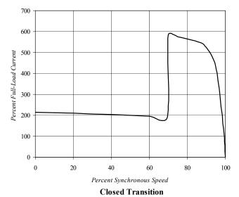
running speed. The high inrush current, especially on large motors, may cause problems with the
