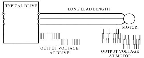
Toshiba EQP III motor designs meet the requirements specified in the 1998 guideline and there are simple guidelines for installing Toshiba motors on drives. Normal wiring methods may be used. No special cable is required except that motor leads be installed in separate conduit and not mixed with other wiring. The following lead length limitations are safe when used with a Toshiba EQP III motor and any Toshiba ASD.
