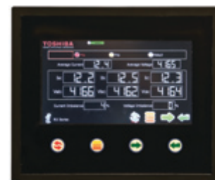
Touchscreen, showing RX Relay display in Spanish.
