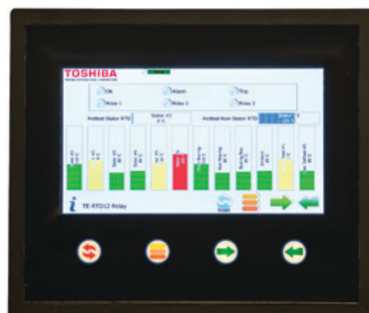
Touchscreen showing TE-RTD Relay with all 12 RTD temperatures.
