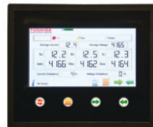
Touchscreen, showing RX Relay display in English.
